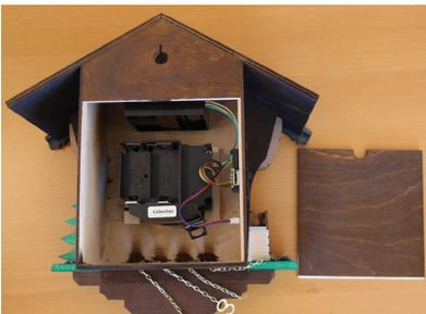
3. Open the back cover and insert two size-C batteries into the battery holder.
